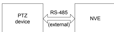
Figure 1. PTZ connection with a NVE
